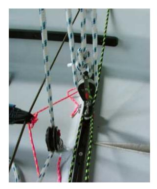
The competitor may also set up the boat with a single traveller car by attaching the single becket block to one of the cars, as in the photo at left, and taping the other car out of the way at the end of the traveller bar.
