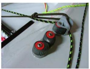
Shock chord may also be used to lift the front of the straps but, if the competitor does this, they shall supply their own additional shock chord. Shock chord at the front of the straps may only be attached to the traveller cleats. See left. **PLEASE NOTE: The cleat configuration at left has been changed**
